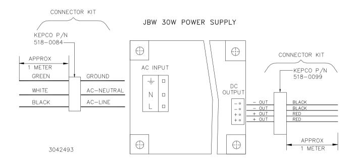
FIGURE 1. CABLE KIT INSTALLATION
